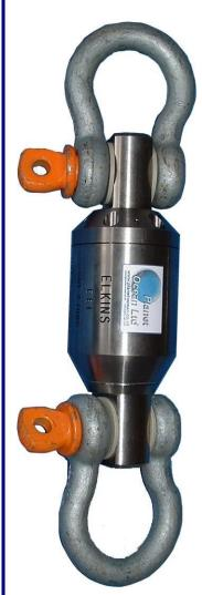
The Elkins EE-1 swivel features a rotating spindle which is located exactly within twin needle roller bearings with the inline forces being carried independently via a single heavy duty thrust race. The complete assembly is oil filled and due to its unique pressure balanced system can ensure freedom of movement even at the greatest ocean depths.
