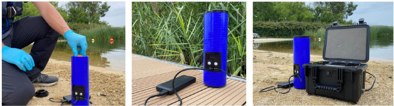
Left sample being loaded into the Alert ONE – Middle Alert ONE performing measurement - Right Performing measurement at urban bathing site.
