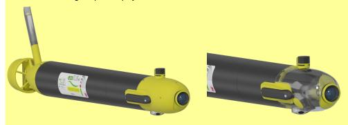
Payload: Valeport CT • Marine Sonic Technologies Scout ARC Mk II Side Scan Sonar (900, 1200, 1800kHz or dual frequency) • ecoCAM 4K camera • Nvidia Jetson Nano Backseat GPU • Nortek Nucleus DVL-1000 (with currents) • Nano-modem (option for Sonardyne AvTrak6)
