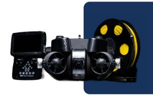
Built with carbon fiber and anodized aluminum that ensures durability in the harshest conditions. Ideally suited for hull inspections, port security inspections, hydroelectric inspections, infrastructure inspections, ocean exploration, and more.
