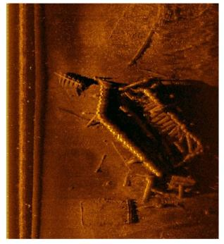
The above image of the *Betsy*, known as YO88 sunk in 1781, Yorktown River, was taken with the ARC Explorer using 1200 kHz transducers at a 40 m Range. The corrugated steel cofferdam is clearly visible around the wreck highlighted by the density of the steel. The less dense elongated concrete blocks protecting the top of the wreck resemble the ship's deck and can be distinguished from the steel.
