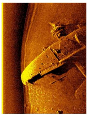
The above image of a WW II era Curtiss SC "Seahawk" float plane found off Iceland was taken with the ARC Scout Mk II using 1800 kHz transducers at a 25 m Range. The details of the engine and underside of the aircraft are clearly visible on the wreck.
