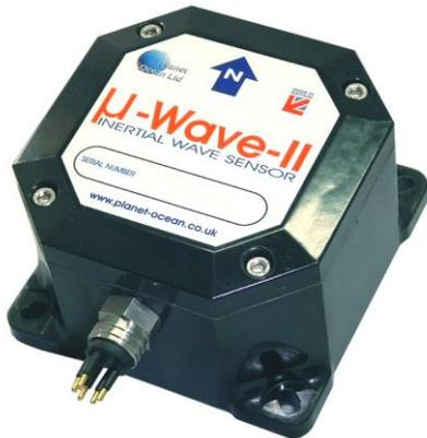
The  $\mu$ -Wave-II Inertial Wave Height Sensor is a +5v to 30v ,low powered (150mW@12v) wave system that reports heading, significant wave height, dominant wave period, dominant wave direction, maximum wave height and maximum period via RS-232. Also available by user selection is, pitch and roll, the first 5 Fourier coefficients and accelerations.
