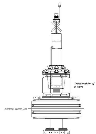
$\mu$ -Wave is housed in an IP-68 enclosure with a 5 pin Impulse connector for power and data.
