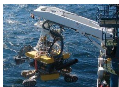
Spider ROV on ORMEN LANGE umbilical survey © StatoilHydro
