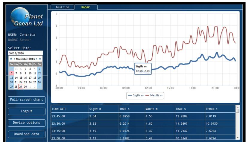
Wave data are sent to a secure web server where they are available on any internet enabled device along with system health information. Users can set alarm thresholds to send email alerts if required. Data are stored within the DBT-3, the RADAC Server as well as the data server.
