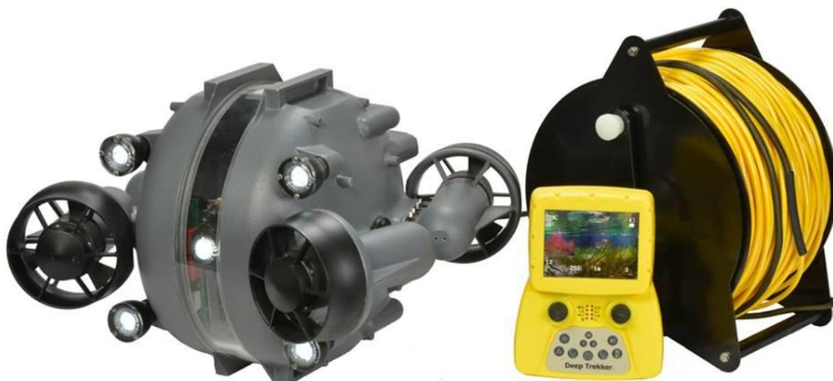
**Built on the proven DTG2 platform, the DTX2 performs in your challenging environments. Depth rated to 305 m with robust vectored thrusters to move laterally and work in currents.**
