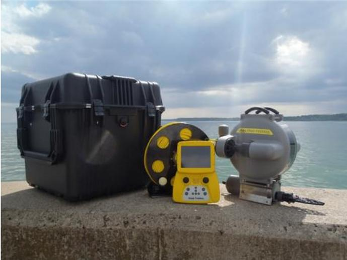
**The DTG2-Worker comes complete with 2 function manipulator-grabber, 100m tether, 125m depth rating robust tether reel, carry case, turbo thrusters and Super Bright Screen Controller with sensor pack for on screen data display and auto depth and heading.**
