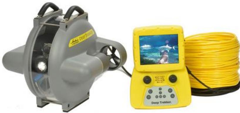
**The DTG2 STARTER model comes complete with a 50 m tether, a 75m depth capability, and now with the Super Bright Screen Controller. For the first completely portable remotely operated vehicle**
